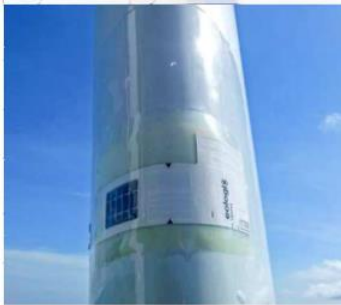
Figure 28: eologix sensor mounted on the leading edge of the rotor blade.
