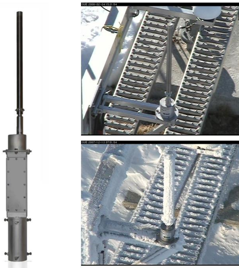
Figure 5: Combitech IceMonitor without (top) and with ice accretion (bottom).
