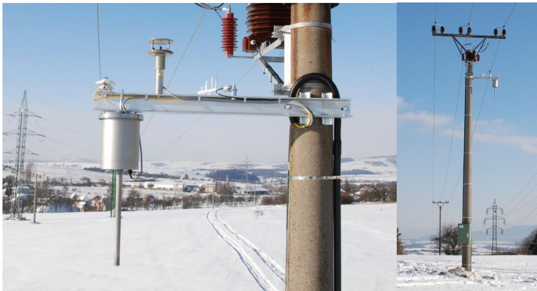
Figure 19: The meteorological monitoring station PMS with the support arm and the sensor with the vertical rod for measuring ice load, temperature and relative humidity. The green central box can be seen on the right.
