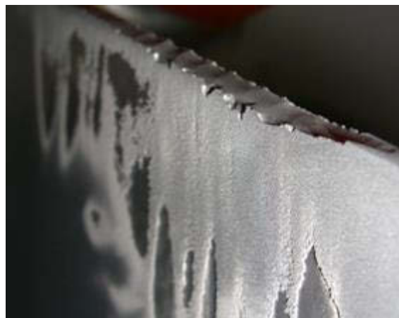
Studying hydro-abrasive erosion, AXPO, Switzerland.
