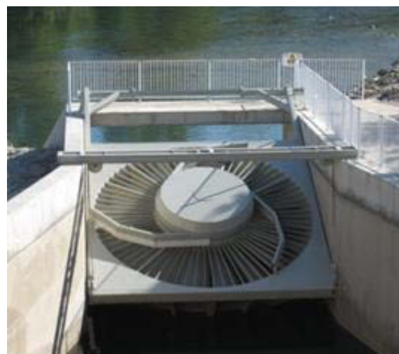
A VLH in lifted maintenance position.
