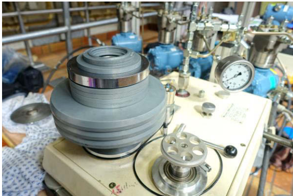
Death weight manometer at HPP Silz, TIWAG, Austria.
