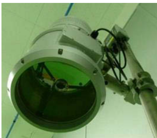
View inside the detector with heated sight glass to prevent condensation
