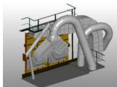
Filter Scan and remodelling Spare Parts are Produced from the Data. of 12x5x6 meter.
