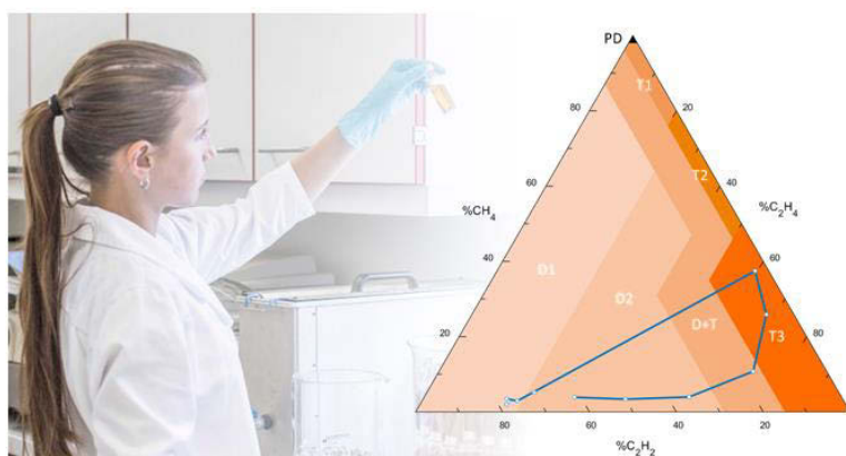
Diagram - An exemplary Duval triangle generated with the data available from historical routine analyses, summarized and evaluated via the innovative VUM analysis tool for insulating liquids. This simplified and quick visualization enables the customer to evaluate the high voltage assets at a glance, indicating the evolution of a thermal fault. In this case, the customer had sufficient time to react upon the possible thread. The efficiency of the repair measures taken is easily visible respectively can be tracked in the analysis tool.
