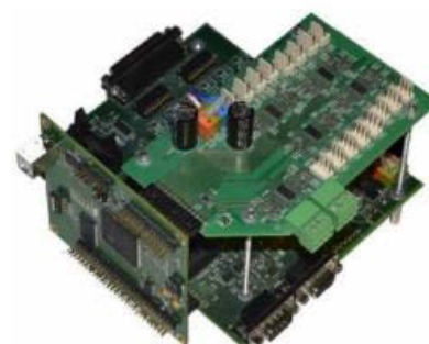
Control system with DSP TMS320F28335 + data acquisition extension.
