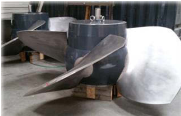
Axial Horizontal Kaplan Runner Ø 2,800 mm 2,000 kW.
