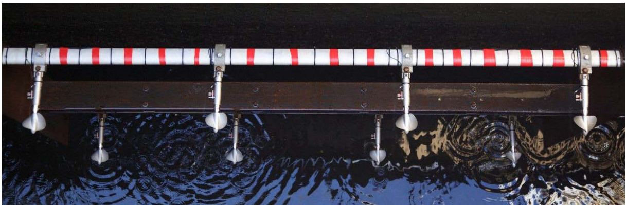
Current-meter measurements at HPP La Rance, EDF, France.
