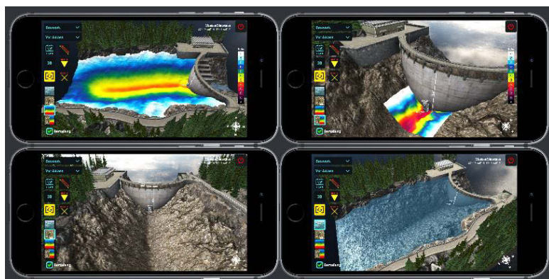
Examples of visualization and analyses of sedimentation at a hydro power dam.
