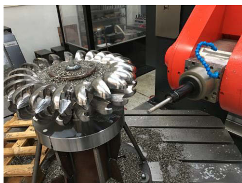
Pelton runner being machined on a 6-axes machine.
