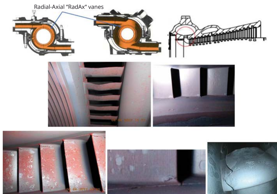
Fig. 3. Radax vanes identification and typical findings
