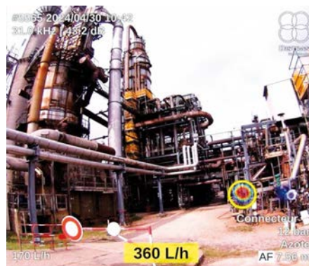
Fig. 3. Ultrasonic detection of a gas leak with a flow rate of 360 L/h measured at approximately 7.5 m and indication on the acoustic frame (right).
