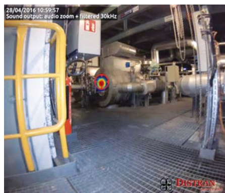
Fig. 9. Superheated steam leak detected at a distance with DISTRAN Ultra Pro X.
