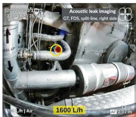
Fig. 10. Methane leak detected in a gas turbine fuel distribution system.
