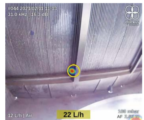
Fig. 8. Vacuum leak on an air-cooled condenser.
